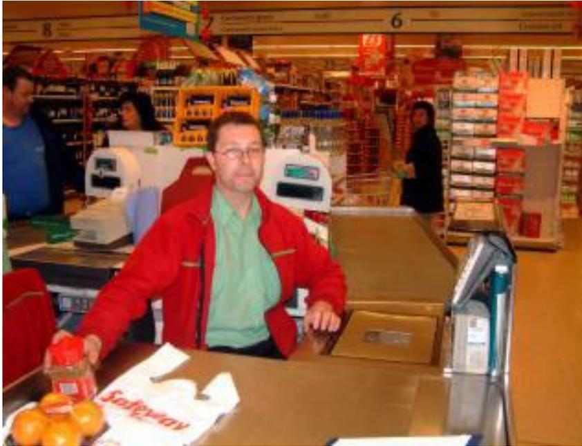
Located at each checkout is an ELECTRONIC POINT OF SALE ( EPOS ) till. This EPOS till comprises a keyboard, a digital display, a scanner which reads bar codes, a set of scales, a printer, a credit / debit card reader and a till drawer. Each till also has its own base to which all of the above is attached. It is the base unit which is connected by cables to the branch computer in the supermarket's system office.
