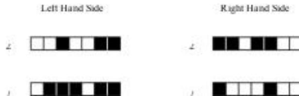
The diagram shows the pattern of lines for each digit on the bar code. Notice that the pattern for a digit on the right hand half of a bar code is the opposite of the one on the left hand half.
