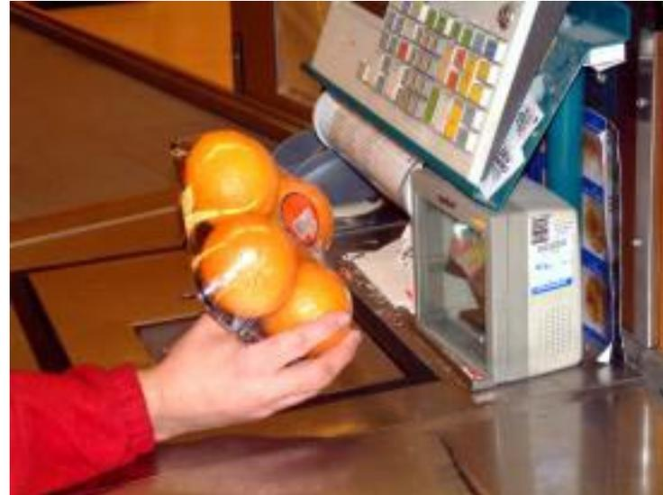
The bar codes on products are read by the EPOS tills at the checkouts. This is achieved by using a scanner, which sends out infra-red laser beams via a set of mirrors, enabling the bar code to be read at most angles.
